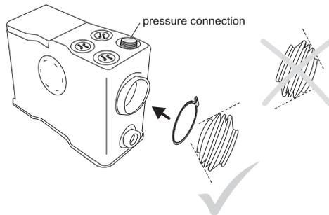
Install sealing sleeve DN 85 (small diameter on the lifting unit – larger diameter on the toilet) with hose clamp 80-100 on the side inlet and with hose clamp 100-130 on the toilet and tighten the clamps.
