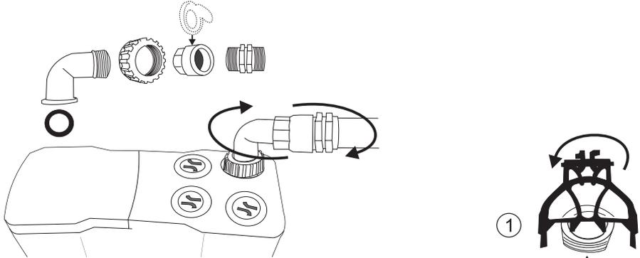
*Pressure line, outlet with 90° elbow,
