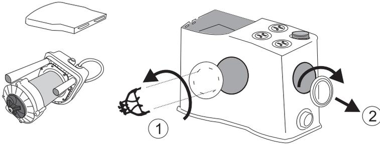
1. ▷ Remove the cover at the front using the special tool
