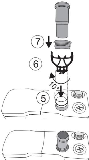
5. ▷ using the special tool, insert the opened inner inlet in the inner groove
