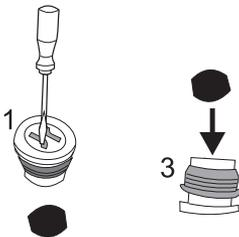
6. ▷ using a screwdriver, press the activated carbon out of the cover no. 1 and place it into the cover no. 3 (not applicable if the venting variant "Venting via the roof" is executed
