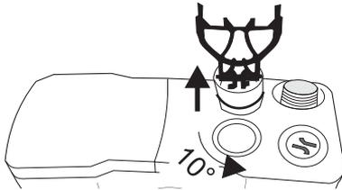
3. ▷ by means of the special tool, now pull out the inner inlet; while doing so, turn the tool in the groove about 10° anti-clockwise (noticeable resistance) and pull upward
