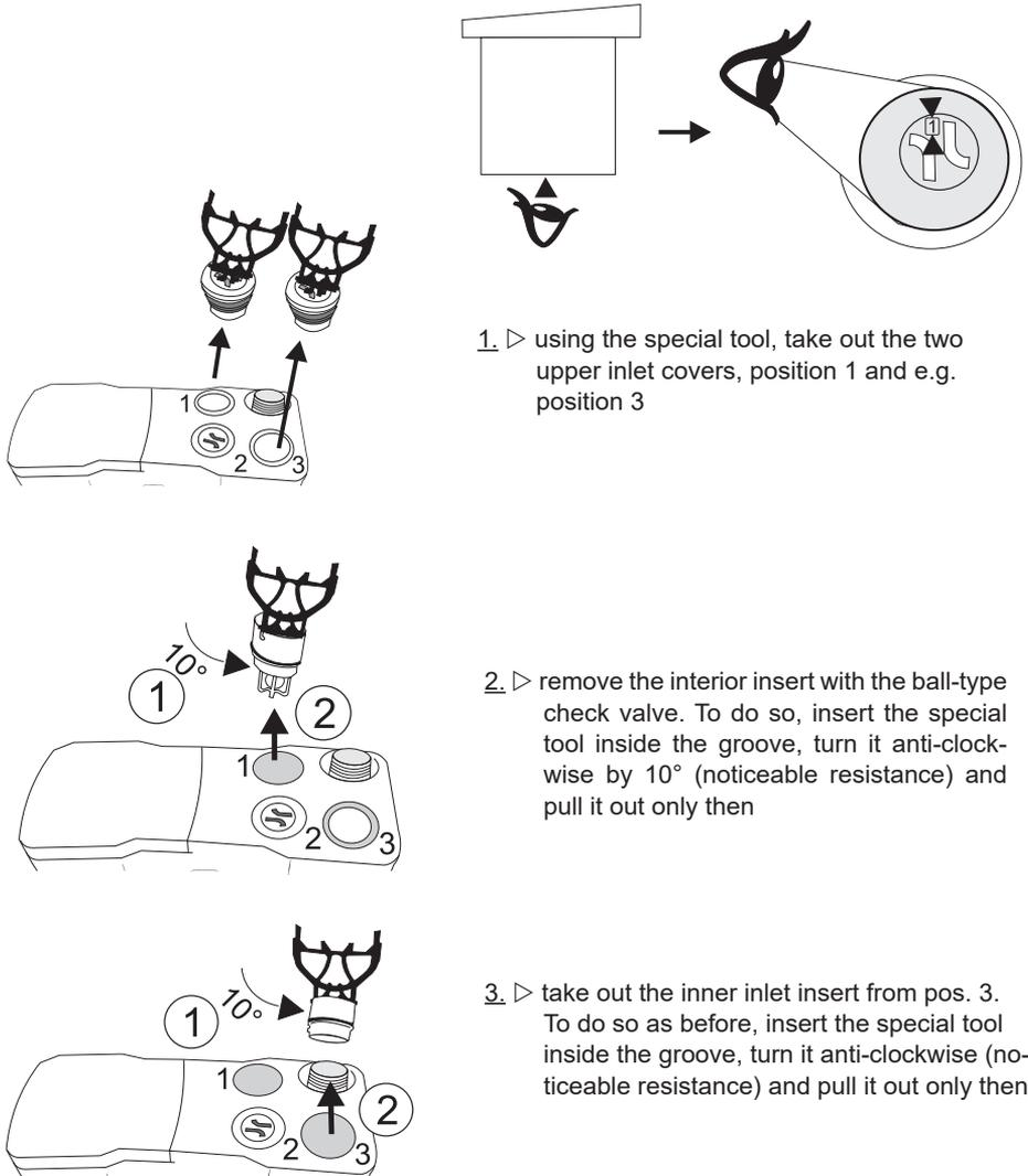
1. ▷ using the special tool, take out the two upper inlet covers, position 1 and e.g. position 3
