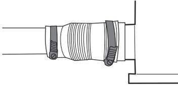
3. ▷ then install the sealing sleeve with a hose clip 40 - 60 on the lateral inlet nozzle, and with a second hose clip 25 - 40, fasten the sealing sleeve and the inlet line of a shower, for example
