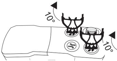
5. ▷ using the special tool, lock both inserts by turning it approx. 10° clockwise (noticeable resistance)
