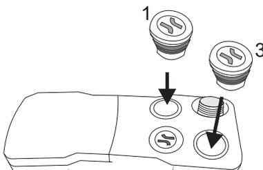
7. ▷ now put the cover no. 1 and the cover no. 3 back to the respective position; when inserting, pay attention to the geometry of the device surface
