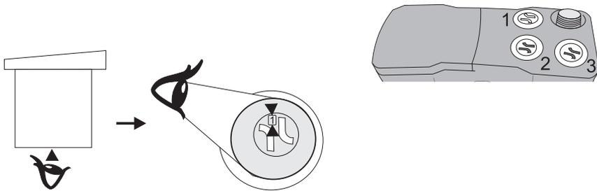
In delivery condition at position 1, there is the ventilation with activated carbon (can be changed ↪ Chapter 5.4.3 “Changing the venting position”)
