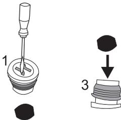
6. ▷ using a screwdriver, press the activated carbon out of the cover no. 1 and place it into the cover no. 3
