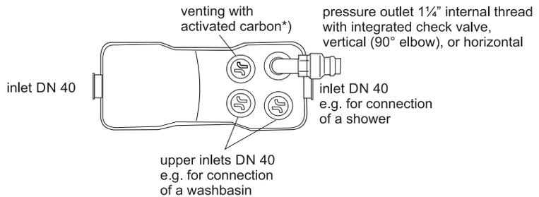
\*) Delivered condition! The inserts can be interchanges as required
