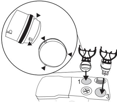
4. ▷ now snap the inlet insert and the insert with the ball-type check valve by a respectively pressing rotary movement using the special tool in the inner groove of the respective opening
