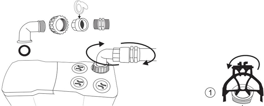
*Pressure line, outlet with 90° elbow,
