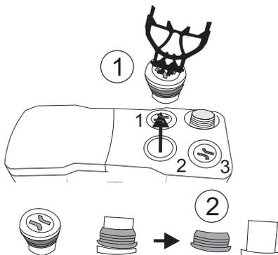
1. ▷ using the special tool, take out the inlet cover, position 2
