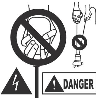
Never pull the power cable or float. It may cause damage to the motor and an electric shock.
